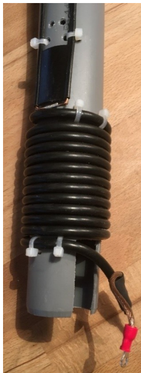
RF choke made with RG-58 wound on a piece of PVC pipe
