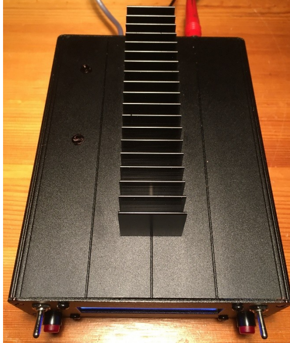
Figure 2: View from above with the well-dimensioned heat sink
