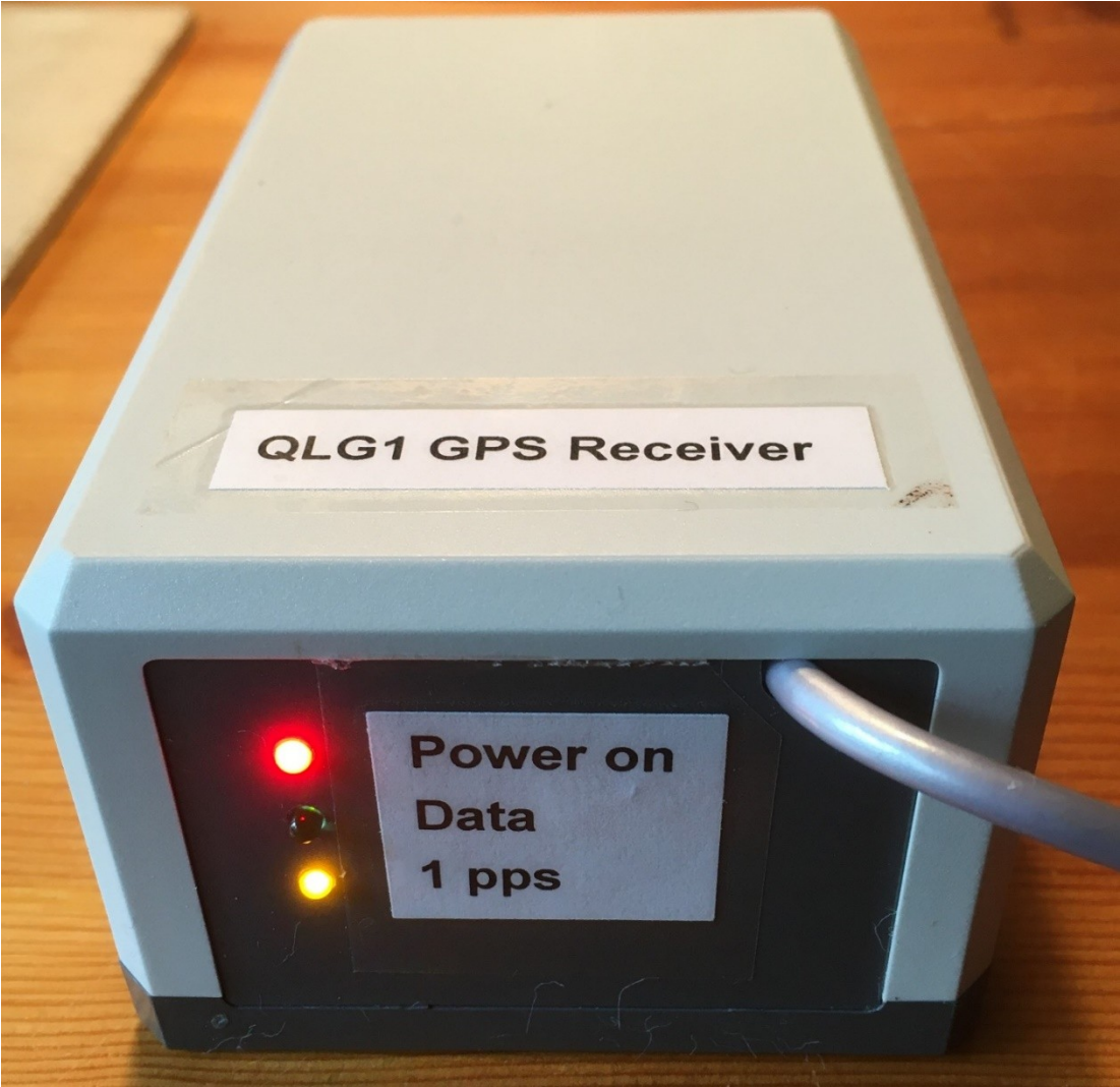
Figure 4: The QLG1 from QRPLabs installed in a separate housing.
