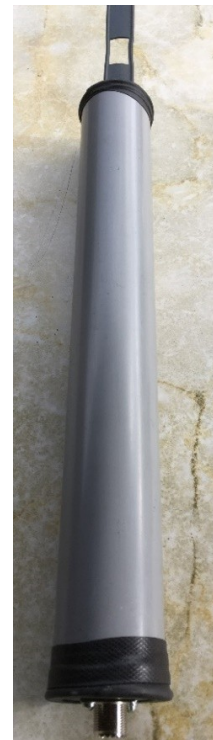
Completed antenna with protective tube covering
