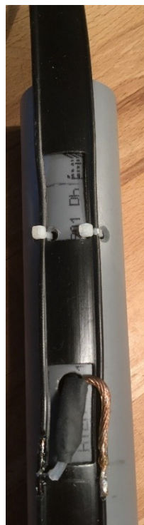
Coax being fed to the 450Ω ladder line
